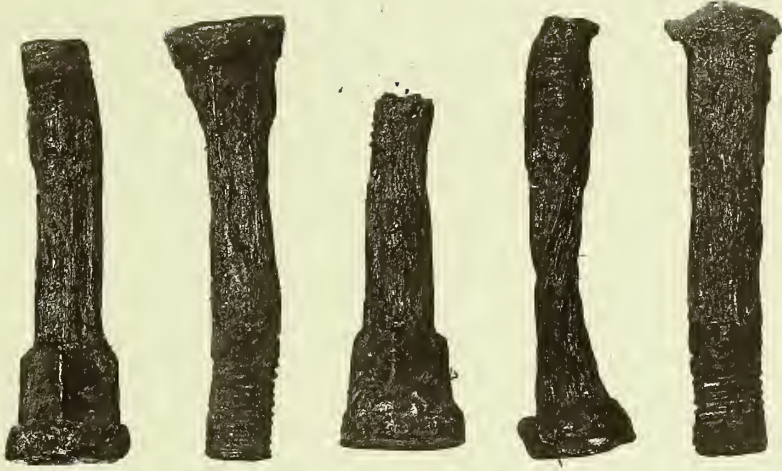
Galvanized Bolts, wasted by chemical action.
